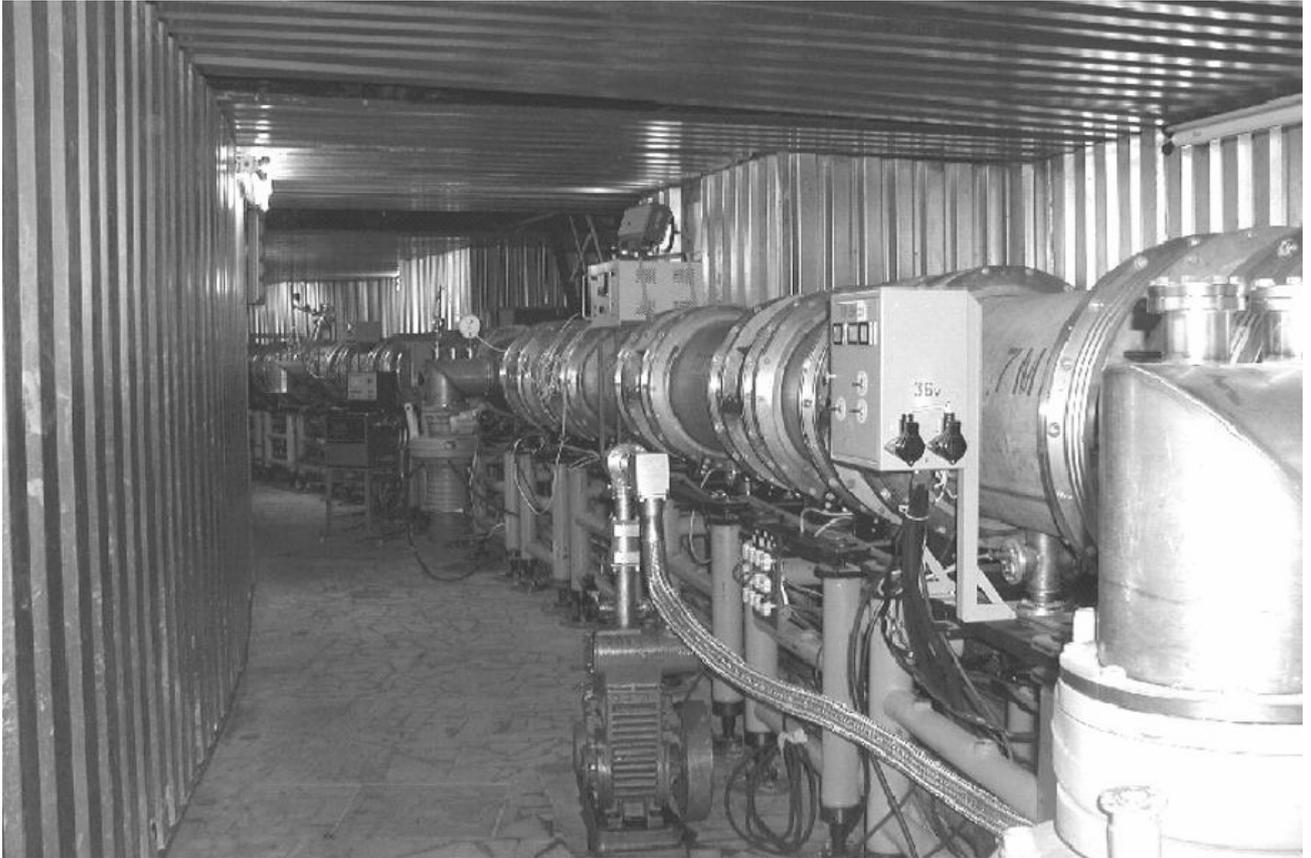
Figure 3 – Photograph of the ring cryostat of the Nuclotron
